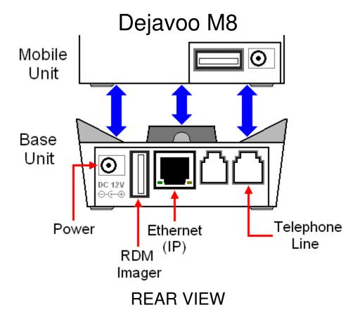
The interconnecting cable is a Standard "A" to "A" USB Cable.
