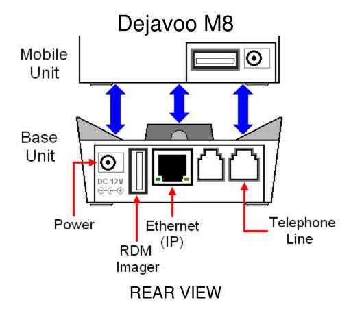
The interconnecting cable is a Standard "A" to "A" USB Cable.
