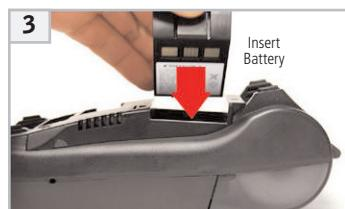
Remove any protective tape that may be covering the battery contacts. Insert the battery module by inserting the left end of the battery into the terminal (as shown). Rotate the battery module into the terminal until the inset latch clicks.
