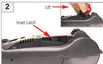
Remove the battery module by squeezing the inset latch on the right side of the terminal (as shown). Lift the right end of the battery to remove (as shown).
