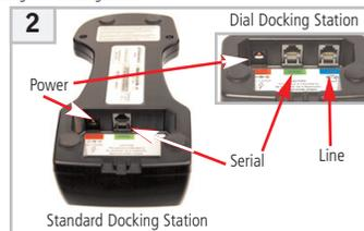
Turn the Docking Station over to display labeled ports:
