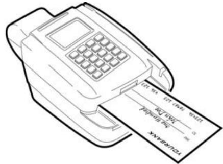
1. Press the latch and lift the cover to access the imaging frame.
